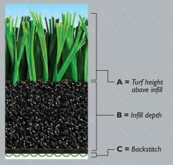
**EPW** =  $\frac{2a}{2a+2b+c}$  **X** Pile Fiber Wt.
